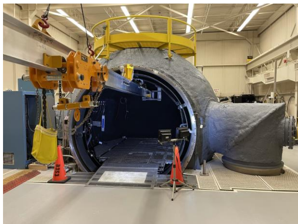
Figure 1: The 15' TVAC Chamber in Building 351
